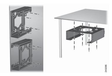
Figure 3-2 Attaching the Mounting Sleeve
